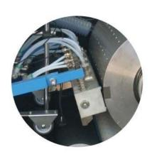
**High speed gluing plotter** for both the "EVA - PSA" hot melt application and vinylic glue. Any shape or design is rapidly glued and prepared for assembly.
